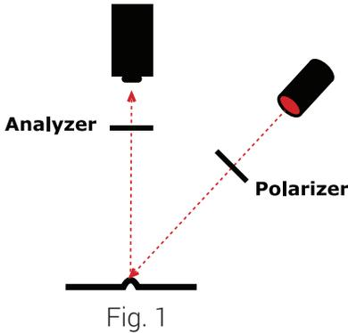
One universal obstacle to quality vision lighting on the plant floor has been unwanted glare, typically from the sample itself, but also from factory ceiling lighting or other dedicated task lighting. We are going to concentrate on reducing glare from the vision lighting, particularly from a sample's curved, specular surface, which is the most common application use for polarizers.
